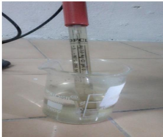
Fig 4.:pH measuring electrode.
