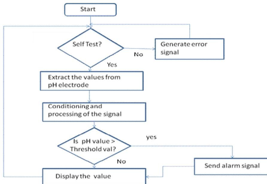
Fig 3: flow diagram of the system
