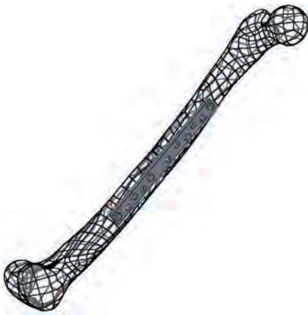
Fig. 10.Assembly of broken bone and plate using SOLIDWORKS
