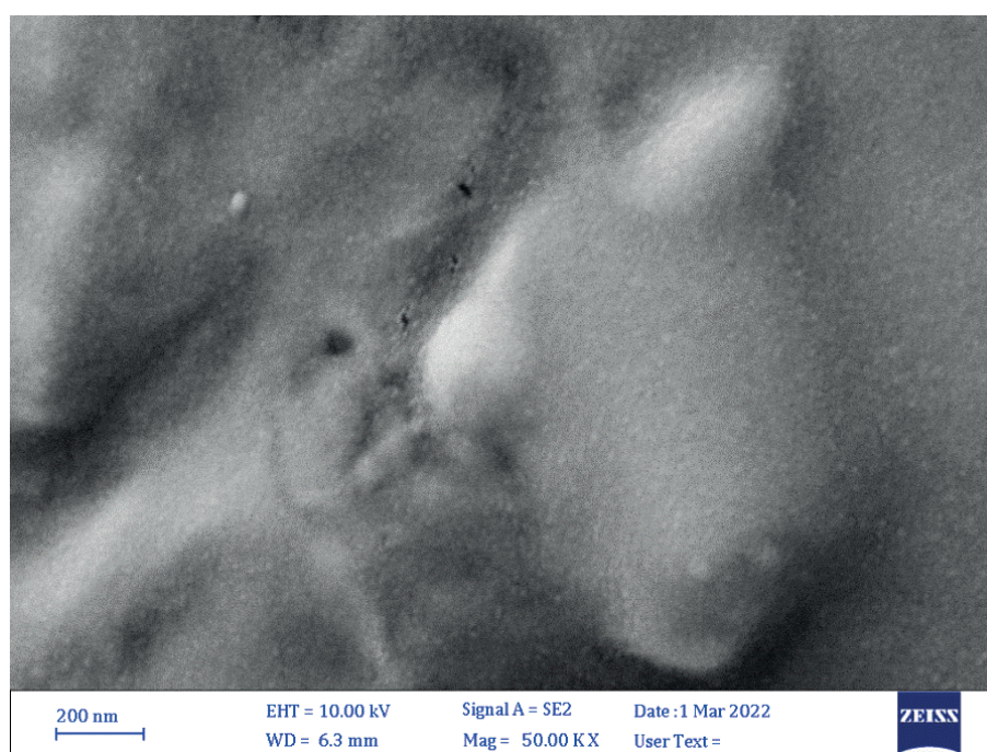
Figure (3): SEM micrograph of biogenic CuO NPs. Size average (16.03 nm).
