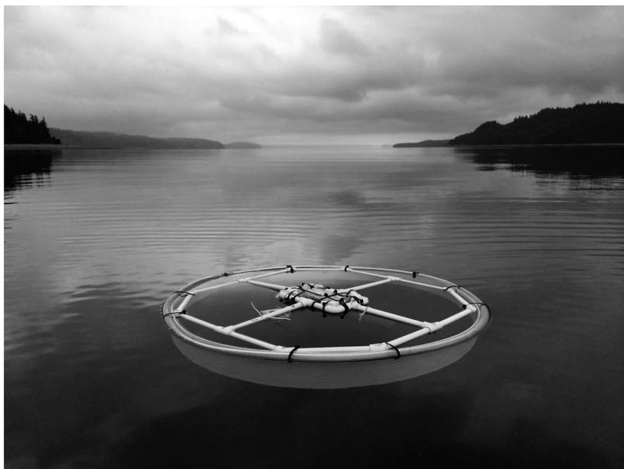
**Figure 2** Neutrally buoyant Lagrangian drifter (diameter 0.8 m), with GPS unit at center. Photo credit: Micah Horwith
