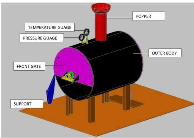
Figure 1: 3D Left side view of composter
