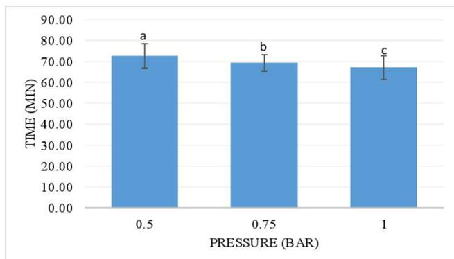
**Figure 6:** Effect of pressure on composting time
