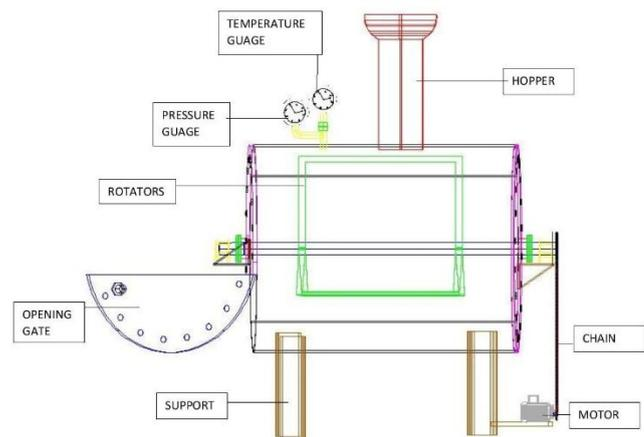
Figure 2: 2D wireframe front view of composter
