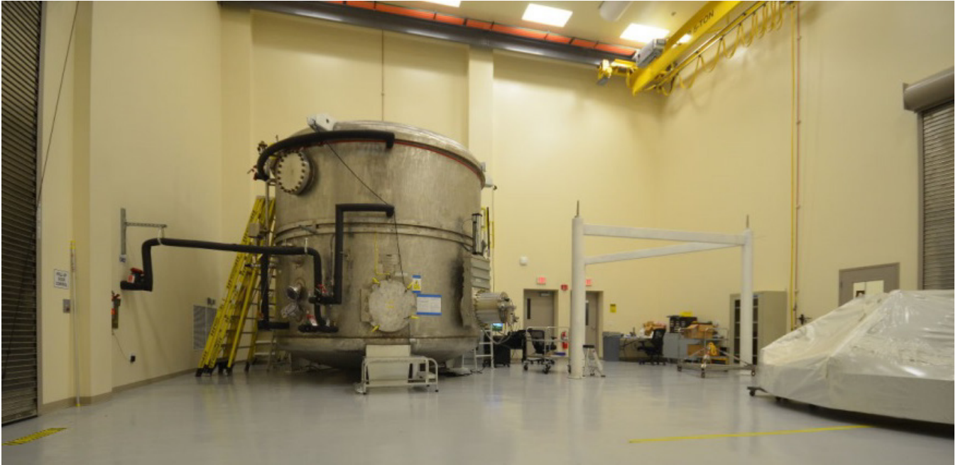
Fig. 5. From the left to the right: the mirror coating chamber, the chamber lid stand, and under the tarp, a mirror weight load surrogate. Also of note are the large bay doors and the overhead crane. A HEPA vent diffuser can also be seen above. Image: Gregory Perryman (USRA).
