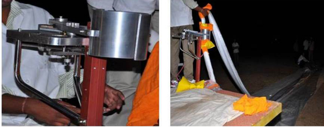
Fig. 7. A close-up view of mechanical launcher (left) and a view of the balloon passing through mechanical launcher (right).
