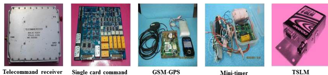
Fig. 6. Control instrumentation packages used in balloon-borne experiments.
