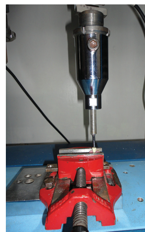
Figure 1: Mounted specimen on universal testing machine for assessing fracture resistance
