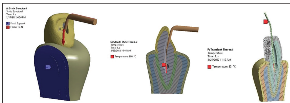
Figure 2: Loading conditions for static structural, steady-state thermal, and transient thermal analysis, respectively
