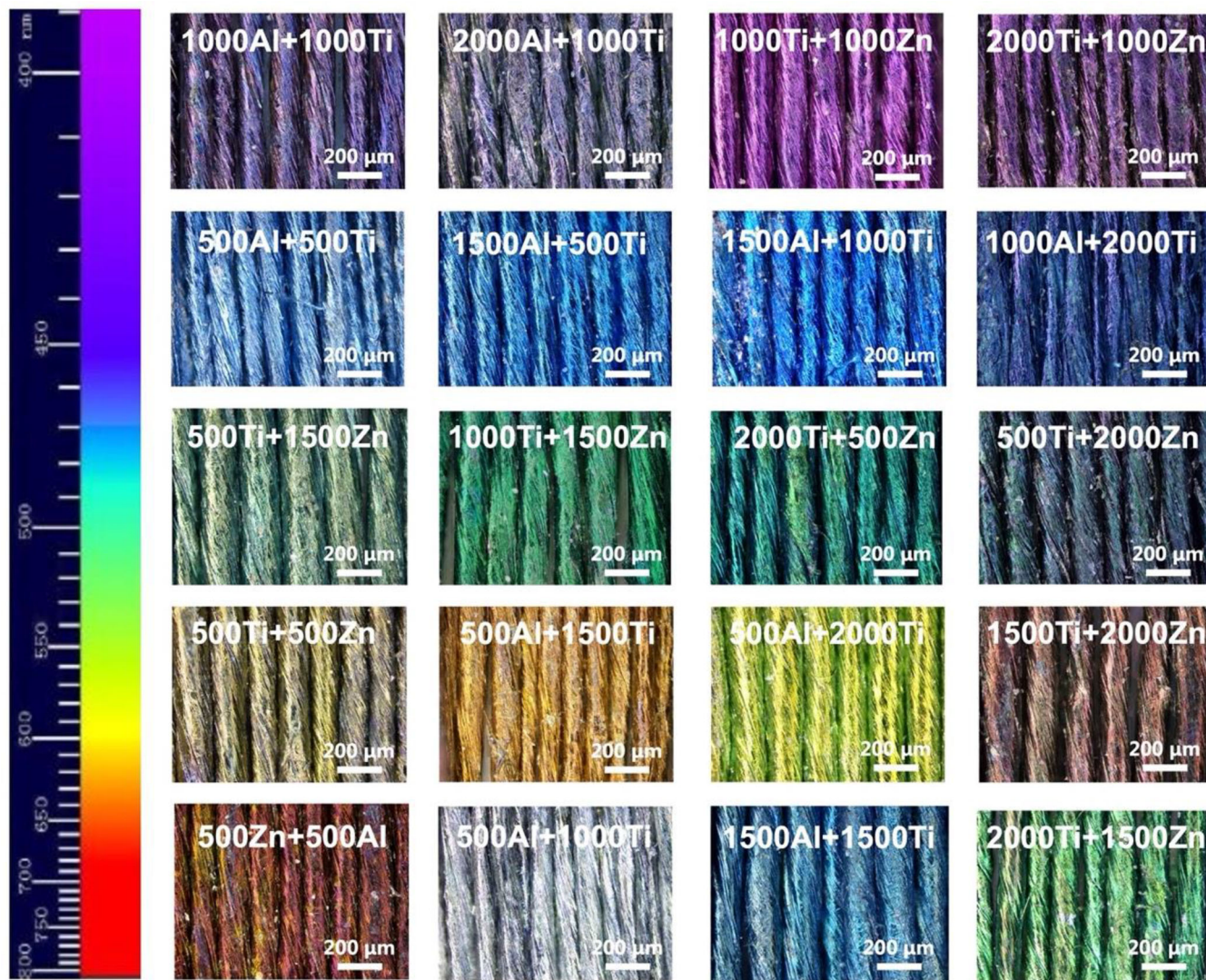
FIGURE 3 Optical images of colored bilayer film-coated CNTFs. Purple, blue, green, and red CNTFs were exhibited from the first line to the fourth line. Red, silver, cyan, and chartreuse CNTFs were exhibited at the bottom line. 1000Al+1000Ti representing the bottom layer is \text{Al}_2\text{O}_3 deposited for 1000 cycles and the top layer is \text{TiO}_2 deposited for 1000 cycles (it is the same case for other similar expressions).
