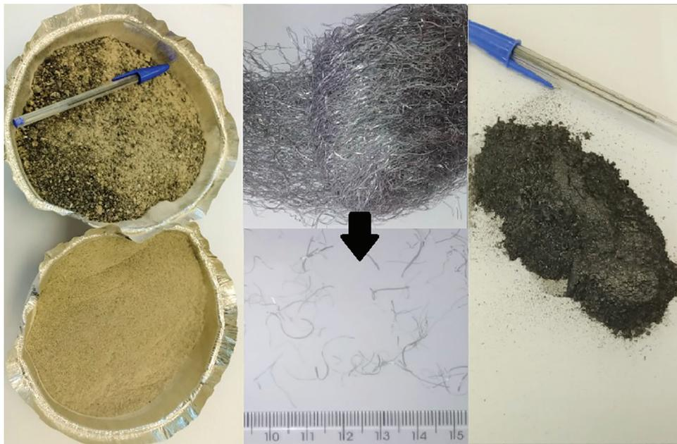
**Figure 1:** Additions used: (a) steel slag before and after grinding; (b) steel fibers in roll and after cutting; and (c) graphite powder.
