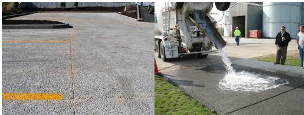
Figure 2. Porous concrete pavement surface and water pouring on surface
