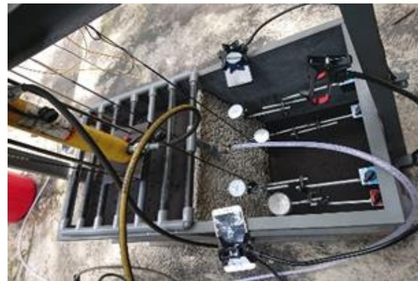
Figure 2. The Installation of Testing Tools Mounted Inside the Test Box
