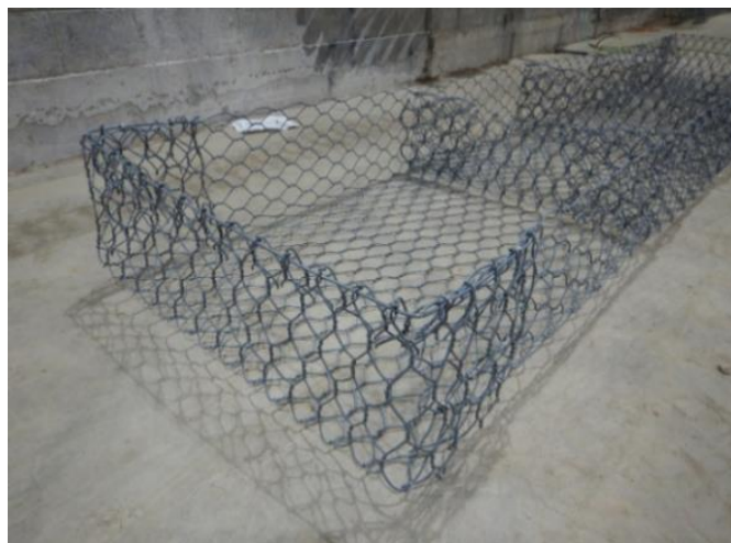
Figure 6. Reno Mattresses unit used during the tests.
