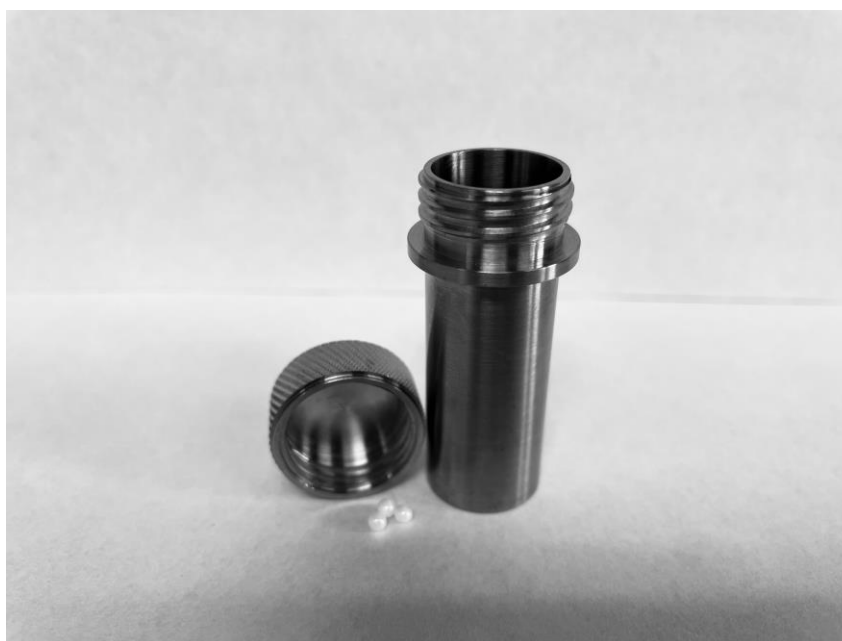
Figure 1. Custom-designed 7 mL stainless-steel tube with ceramic microbeads.
