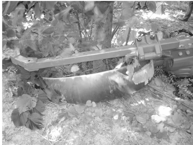
Figure 1. The semicircular blade during the cutting of a root ball. The blade is supported by the frame of the tree digger machine.
