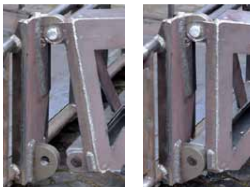
Fig. 10. DATEFF attachment system to the support frame.
