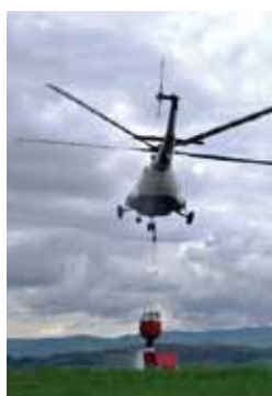
Fig. 8. Filling the DATEFF tank with a helicopter.
