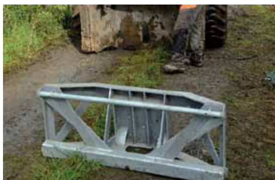
Fig. 9. Mounting of the supporting frame to LKT's rear log arch.
