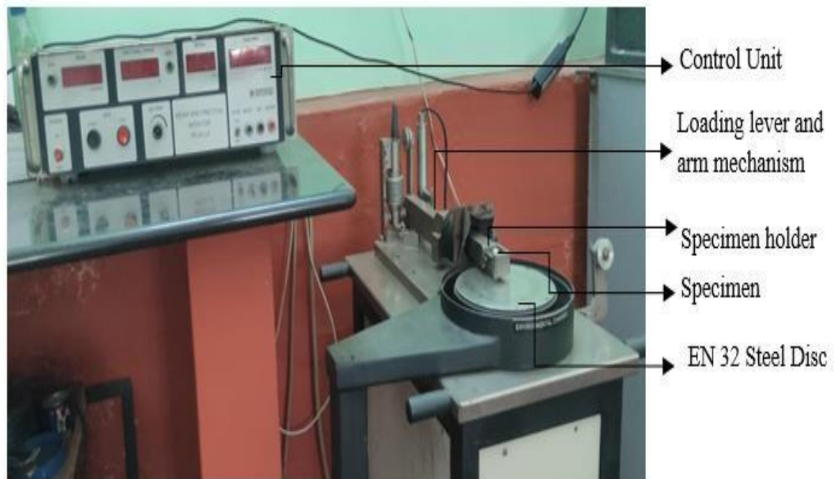
Figure 2. Pin on disc apparatus
