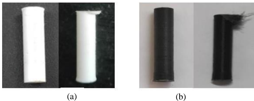
Figure 8. Samples for PLA and CF-PLA composite (a) Before test, (b) After test
