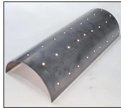
Figure 3. Curved part after isothermal hot stamping.
