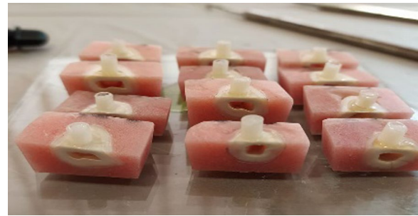
Fig. 1 Insertion of resin composite into plastic molds for bonding to dentin
