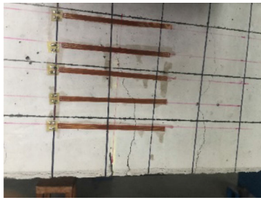
Fig. 4 Site layout of mid-span strain gauge at plane C of track slab
