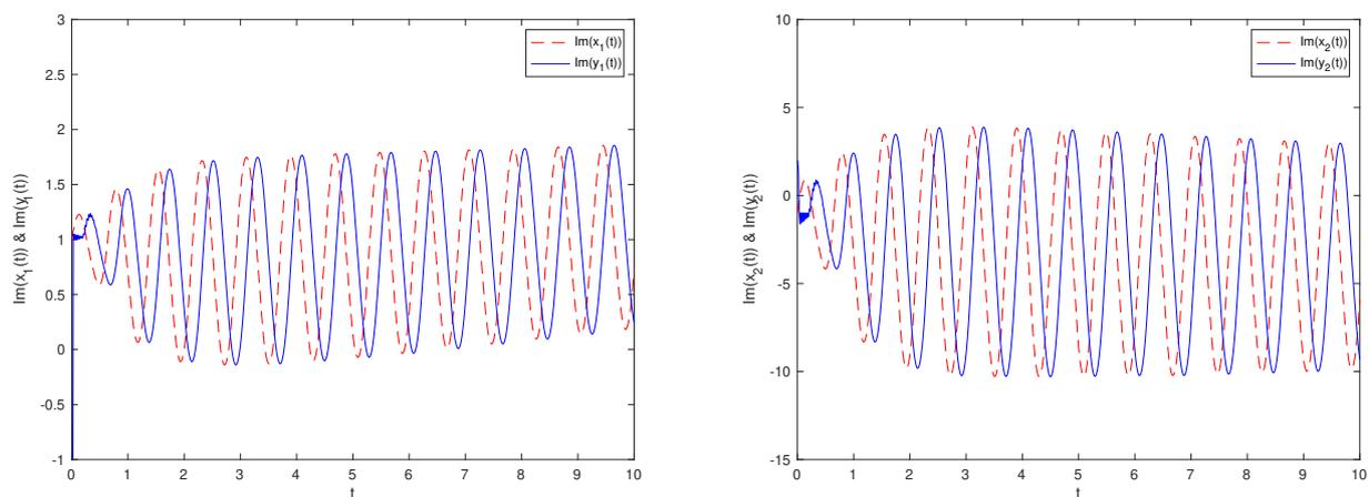
**Figure 4.** State trajectories of imaginary parts of the drive system (2.1) and the response system (2.2) with impulsive control ( $\alpha = 0.2$ ).
