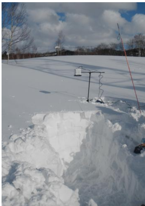
Fig. 1 Snow pit and loudspeaker for acoustic measurement.
