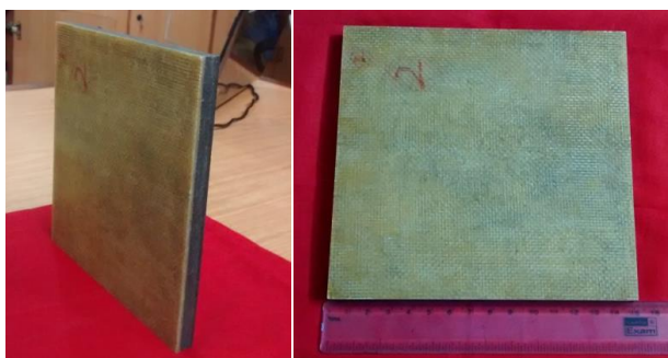
Fig. 12: Free space measurement technique samples of 150\text{ mm} \times 150\text{ mm} in different views
