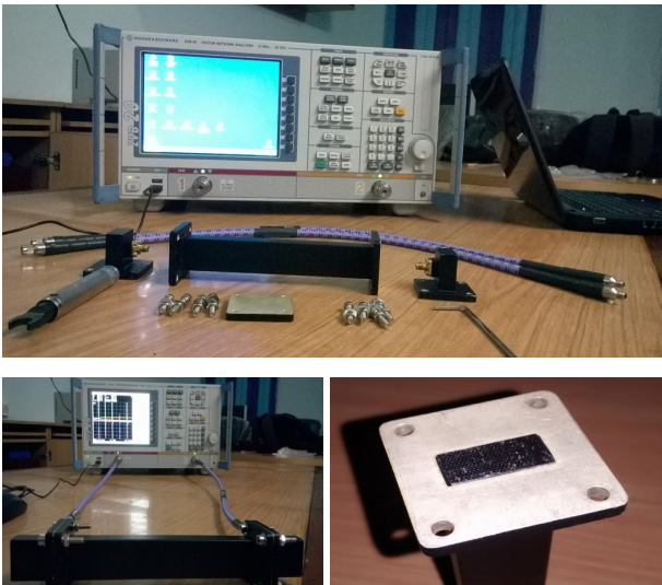
Fig.2: Waveguide measurement setup and sample in X band wave guide
