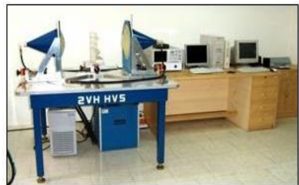
Fig.13: Free space measurement setup
