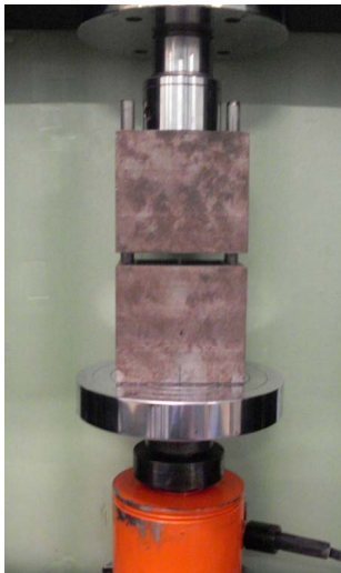
Fig. 1: IITRI compression fixture
