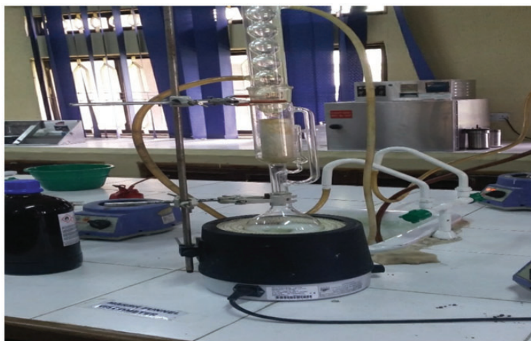
Figure 2. The reflux method set-up for the study.
