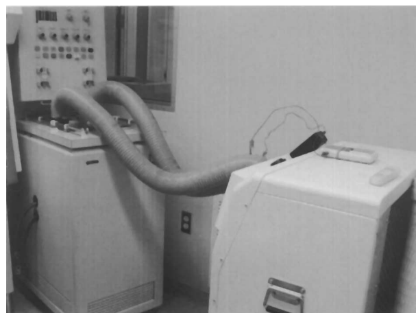
Figure Air-cooled COBE 2991 with Broughton air conditioner connected to the perspex lid above the centrifuge bowl with wide hoses containing temperature probes.
