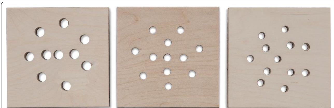
**Fig. 2** The boards of the wooden box. Holes with diameters of 18, 13 and 10 mm
