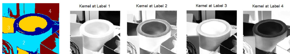
Fig. 5 Left: the example of the initial object label is based on K-mean clustering, in which the number of labels is set to 4. The initial label is not smooth and consistent, so it is converted via RBF kernel function to a higher dimension of four different images in which the distribution of each kernel is changed based on each label characteristic
