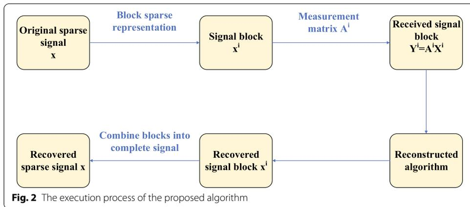
algorithm. The entire process is depicted in the Fig. 2. As shown in the figure,  $x$  is the original sparse signal and  $\hat{x}$  is the recovered sparse signal. By comparing  $x$  and  $\hat{x}$ , the BER performance of the proposed method is obtained.
