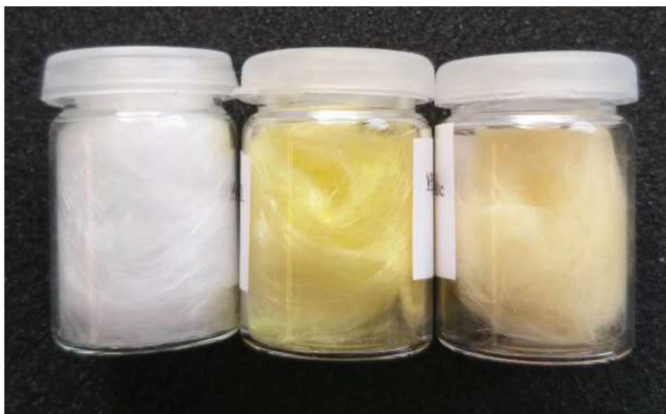
Figure 1. A photograph of the uncoated glass wool, as-deposited samples, and crystallized samples (from left to right). The yellow color is characteristic of \text{UiO-66-NH}_2 .
