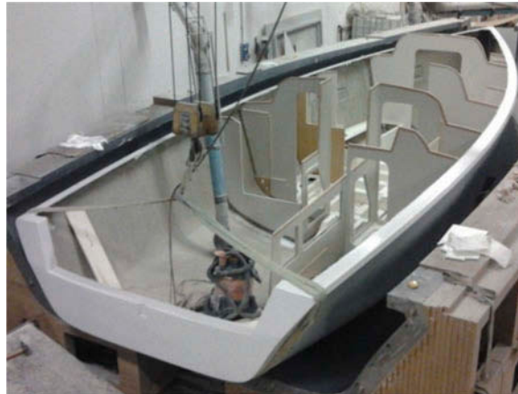
Figure 8. The bulkheads junction to the hull by means of manual layered VTR reinforcement.
