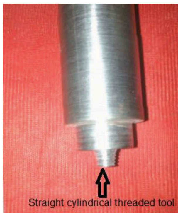
Figure 2. Straight cylindrical threaded tool.
