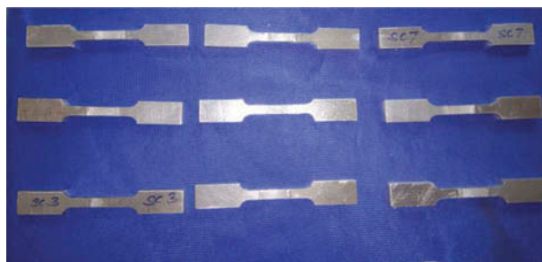
Figure 4. Specimens of the tensile test as per ASTM E8.
