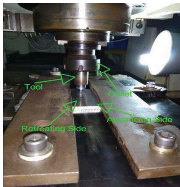
Figure 3. Dissimilar weld position of friction stir welding.
