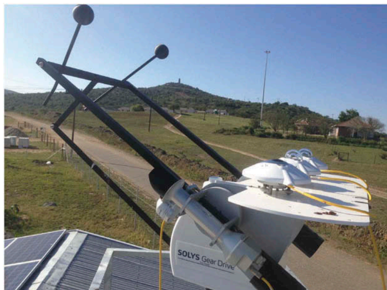
Figure 9. SOLYS gear drive dual-axis sun tracker containing various radiometers.
