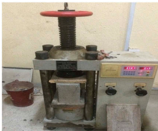
Plate 6. Compression testing machine loaded with sample.
