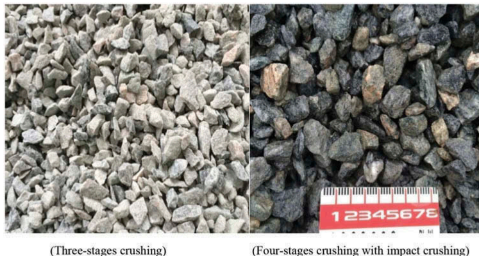
Figure 3. Particle shape change of aggregate by different crushing processes.
