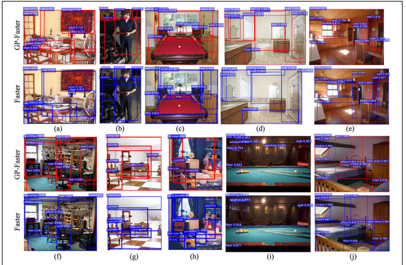
Figure 4. (a–j) Detection examples of Faster16 and GP-Faster16 on the SUN2012 test set. A score threshold of 0.6 is used to draw the detection bounding boxes. The blue and red colors, respectively, show the detections launched by Faster16 and GP-Faster16.
