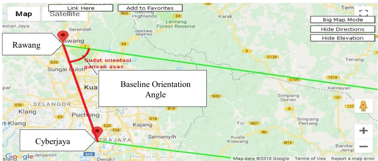
Fig. 2 Baseline orientation angle, an angle between azimuth line (green line) and baseline direct distance of Cyberjaya and Rawang
