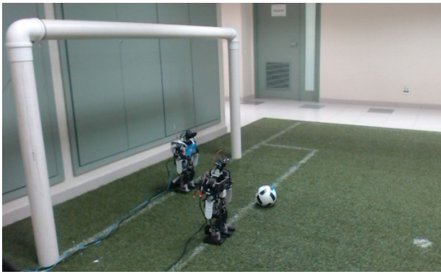
Fig. 1 Two humanoid robots used in the experiments: the Goalkeeper (on the goal line) and the Defender
