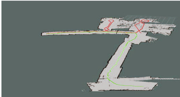
(b) Resulting map of the real world experiment including the trajectories of the two individual robots
