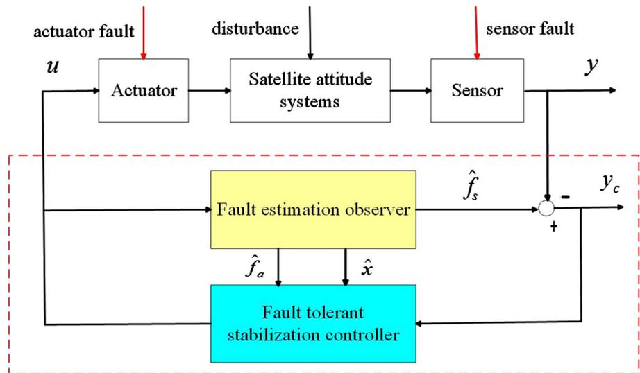
an integrated fault-tolerant stabilization control scheme is developed for the attitude systems of rigid satellite with both actuator and sensor faults in this paper, and the block diagram of FTC is shown in Fig. 1.
