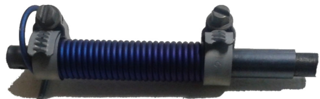
Fig. 2 Fabrication of the SMA actuator
