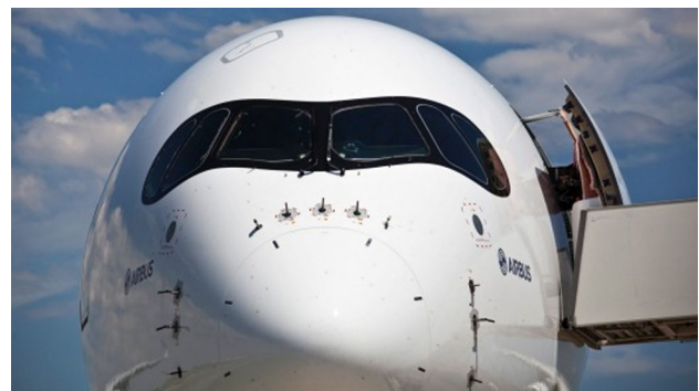
Fig. 2 Airbus A-350 Airdata Systems
