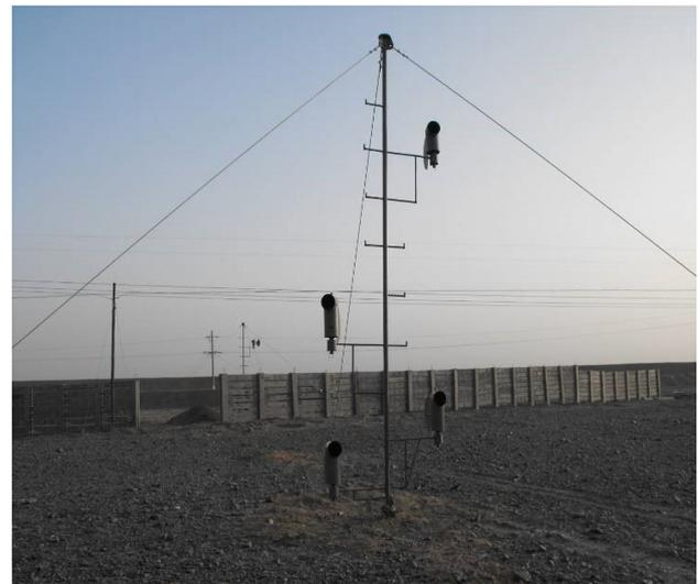
**Fig. 5** Spin-type sand collecting instruments along the LWHR
