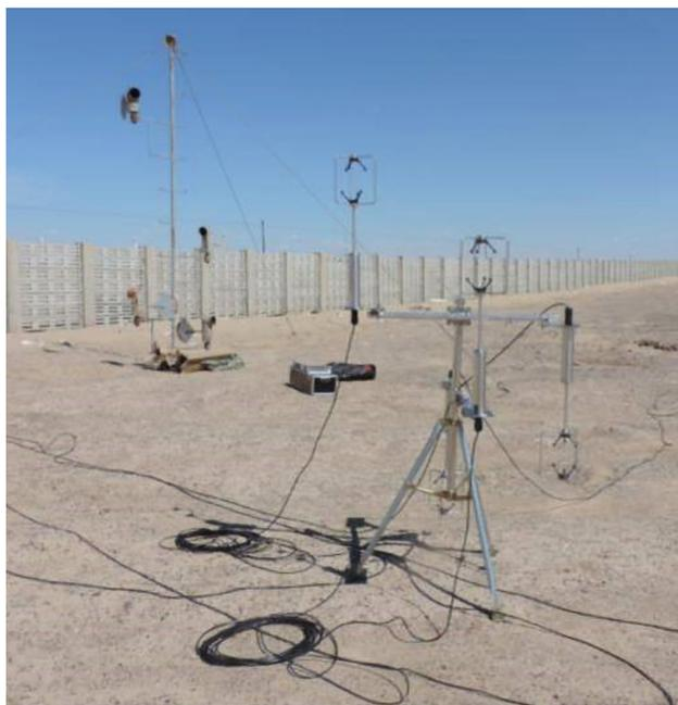
**Fig. 6** Wind Master Pro 3D anemometer for measuring wind speed around fences
