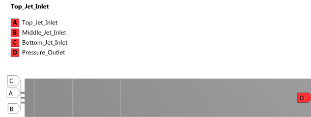
Figure 4: The boundary conditions for confined space
