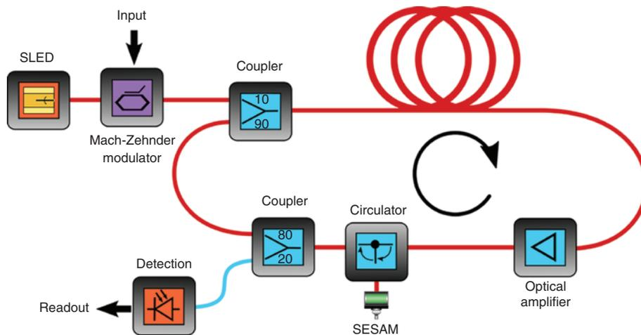
**Figure 10:** Scheme of the all-optical reservoir computer based on the saturation of absorption. The input optical signal is injected into the ring cavity by means of a fiber coupler. The cavity itself consists of a fiber spool used as a delay line, an optical amplifier, a circulator, and a SESAM. A fiber coupler is used to send 20% of the cavity intensity to the readout photodiode.
