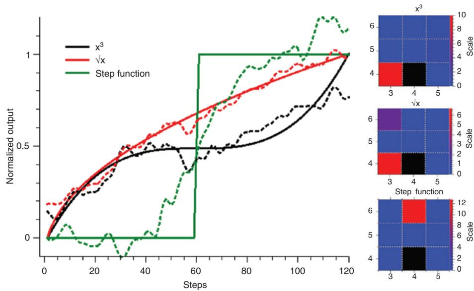
**Figure 5:** Several nonlinear transformations were synthesized from the network of eight injection locked lasers [24]. The y axis corresponds to rescaled values of optical intensities, the x axis to sample points of the input signal (sampling time 100 ps). The right panels show the numerically implemented readout weights of each individual laser.
