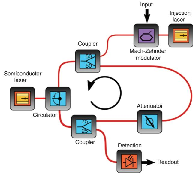
**Figure 9:** Scheme of the all-optical reservoir computer based on a semiconductor laser subject to delayed optical feedback. The experimental setup comprises the laser diode, a tunable laser source to optically inject the information, a Mach-Zehnder modulator, an optical attenuator, a circulator, couplers, and a fast photo diode (PD) for signal detection.
