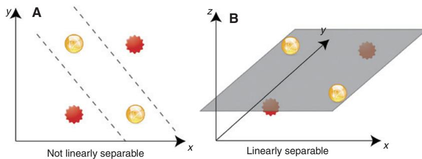
**Figure 2:** Illustration of the operation principle of reservoir computing. In its original  $(x, y)$  representation, two different classes of data cannot be linearly separated (left panel). Upon adding an additional dimension,  $(x, y, z)$  representation, a linear separation via a linear hyperplane can be found. Reservoir computing is based on the creation of additional dimensions to provide such hyperplanes. Figure adapted from Appeltant et al. [20].
