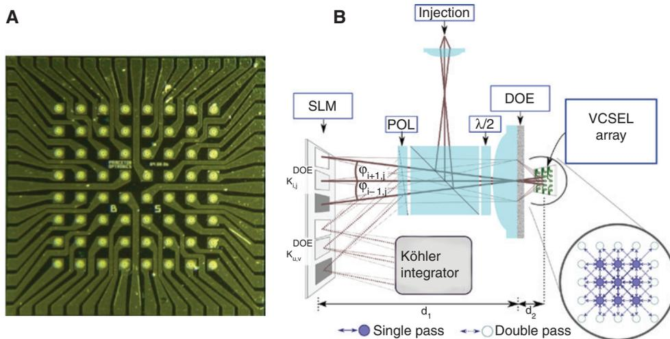
**Figure 4:** (A) Array in single-mode VCSEL laser diodes, Princeton Optronics. Implementing such an array in a diffractive resonator design creates coupling between individual lasers (panel B) [24]. Such a network can then be injected via a single external laser; readout weights can be implemented via a SLM.
