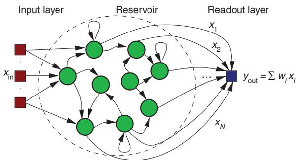
**Figure 1:** Standard layout of a reservoir computer, comprising an input layer (red), the reservoir (green) with randomized but fixed connections, and the linear readout layer (blue). Here, for simplicity a one-dimensional readout layer is drawn ( $l=1$ ).
