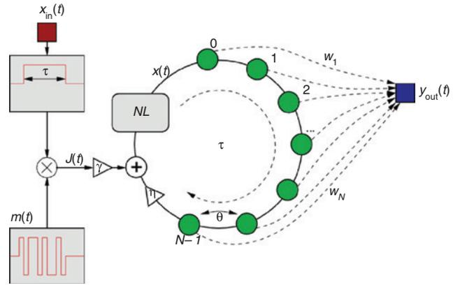
**Figure 6:** Structure of a delay line based reservoir computer. A one-dimensional input signal (in red) is first preprocessed using the masking function  $m(t)$ . Virtual nodes are defined along the delay line and form the reservoir (in green). The output layer (in blue) is unaltered from the standard RC structure.
