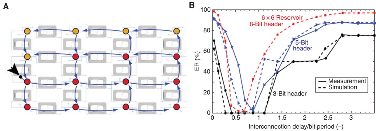
**Figure 3:** Reservoir implemented on a passive silicon chip [38]. (A) A linear optical network is implemented using optical waveguides, splitters, and combiners. Blue arrows illustrate the implemented reservoir connectivity. (B) Experimental and numerical evaluation of optical header recognition via on-chip RC (figure courtesy of Peter Bienstman).
