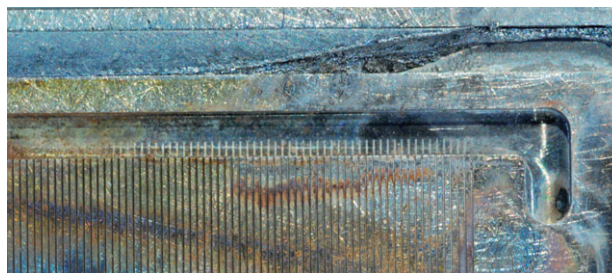
Figure 10 Magnified view of evaporation channels used. Microstructures are intact and not blocked, while some removable flash rust can be seen on the surface.
