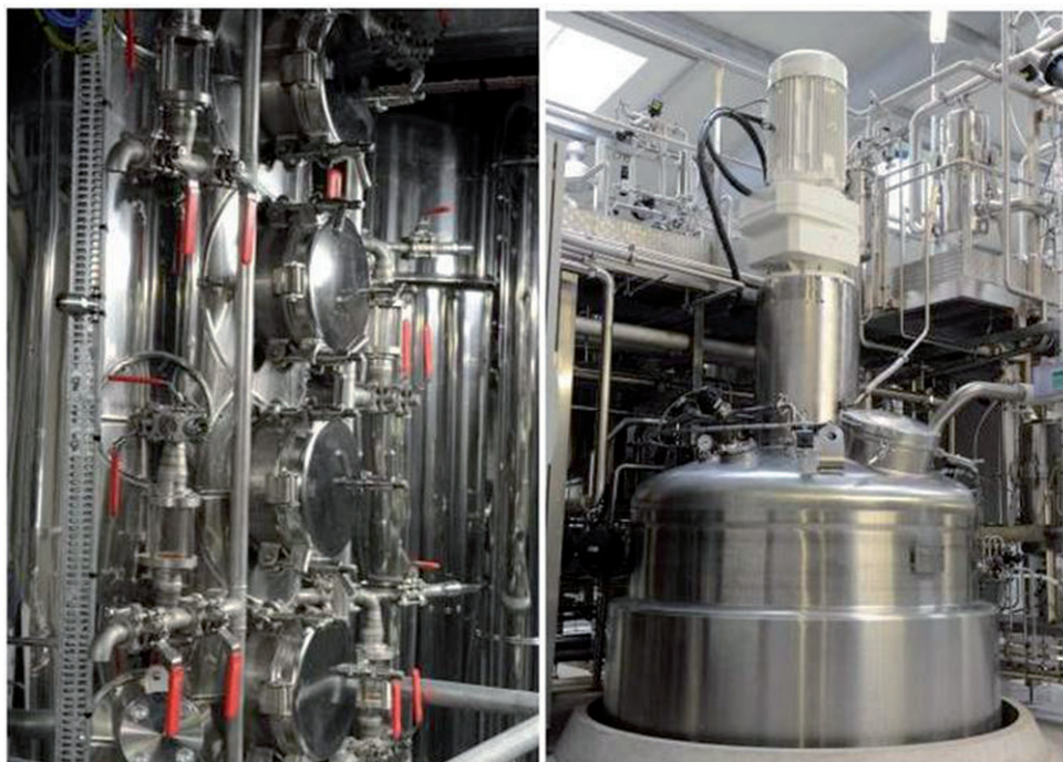
Figure 2 The Futurol project (Pomacle-Bazancourt, France): ethanol distillation tower (left side) and enzyme production (right side).
