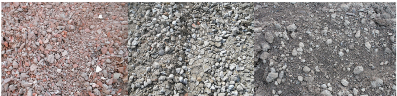
Figure 1: Samples of recycled bricks, recycled concrete, and soil with aggregates.
