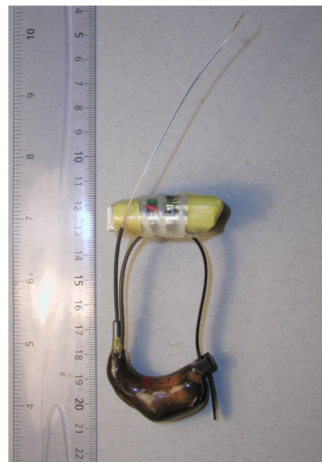
Figure 2. Complete GPS radio collar ready for fitting.
